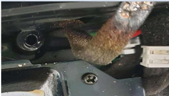
FFC cable melted
