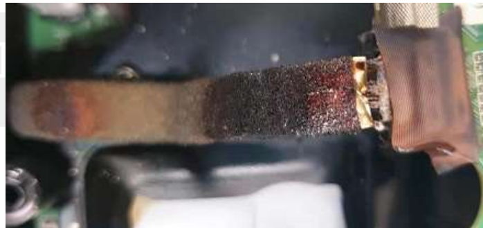
FFC cable melted
